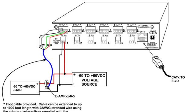
to 1000 foot length with 22AWG stranded wire us the crimp-on wire splices supplied with the E-AMPxx-6-5, E-AMPxx-SC21, or E-AMPxx-SC12.
