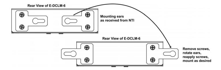
Note: The E-xD must be running firmware version 2.37 or later in order to use the E-DCLM-6 with it. Refer to the E-xD manual for firmware upgrade instructions as needed. To mount multiple E-DCLM-6 in close proximity to the E-16D, install an extension rail kit (NTI E-RL-16D - sold separately) and mount E-DCLM-6 as seen in the illustration below.
